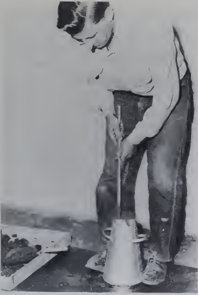
Rodding and filling cone using three separate layers of concrete
